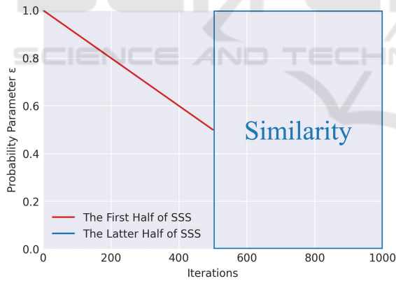
Figure 4: Scheduling strategy of similarity-based scheduled sampling. We propose similarity-based scheduled sampling that utilizes the similarity calculated from the difference frames between the predicted future frames and the ground truth future frames and incorporates this similarity into the scheduling at each iteration. The first half of the training uses scheduled sampling, while the latter half utilizes similarity-based scheduled sampling.
