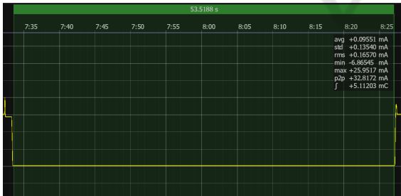
Figure 5: Sleep mode duration between two cycles, highlighting the minimal power consumption of the collaborative node during idle periods, with an average current of \bar{I} = 0.095 mA.
