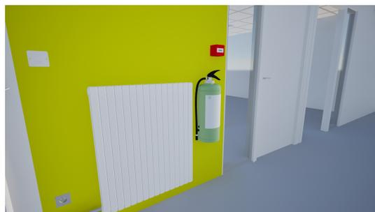
(a) Example of modeled 3D systems: fire alarm, fire extinguisher, heater, outlet, light switch.
