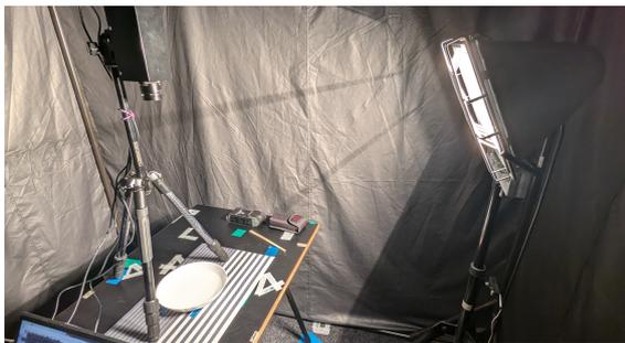
Figure 2: Scene of dataset capture: HS camera positioned above dishes containing water samples.
