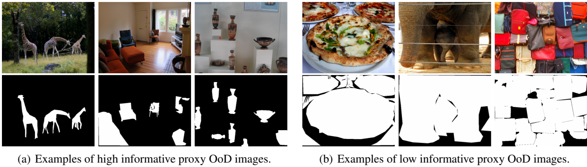
Figure 2: Examples of high and low informative proxy OoD images. The first row contains the proxy OoD images while the second row contains ground truth segmentation masks such that the white regions represent pixels labeled as OoD for which Eq. (4) is applied.
