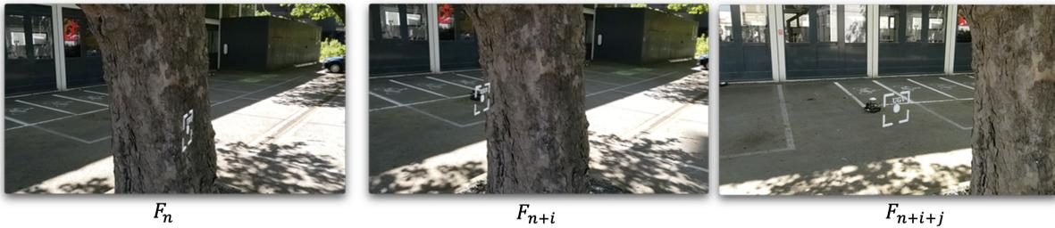
Figure 1: Tracking UGV using RTK systems.  $F_n$ ,  $F_{n+i}$  and  $F_{n+i+j}$  are captured frames from Microsoft HoloLens v2. The white virtual rectangle refers to the RTK information derived from RTK rover system located on UGV. A detailed demonstration of the experiment setup is available in the video: <https://youtu.be/cqJEJmuMtsg>.
