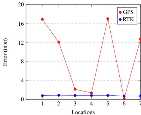
Figure 7: Scatter plot illustrating the errors in distance measurements for several UGV locations obtained using both RTK and GPS systems.
