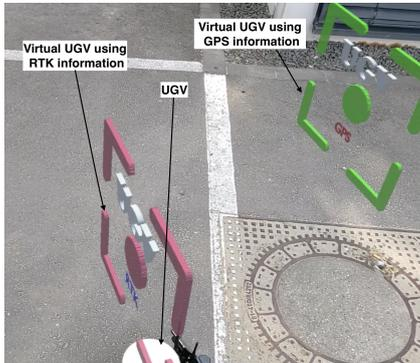
Figure 6: Tracking a UGV using RTK and GPS. Frame is captured from HoloLens v2. The virtual objects (rose and green rectangles) should be in the same position as the UGV such that the green rectangle represents the GPS value derived from the iPhone, and the rose rectangle represents the RTK value derived from RTK rover.
