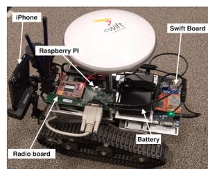
Figure 3: UGV consists of an antenna, Swift Navigation Piksi board, Radio board, battery, phone holder, iPhone 11 Pro, and Raspberry Pi, which is hidden by a radio board that receives the correct position of the UGV using information derived from the RTK station.
