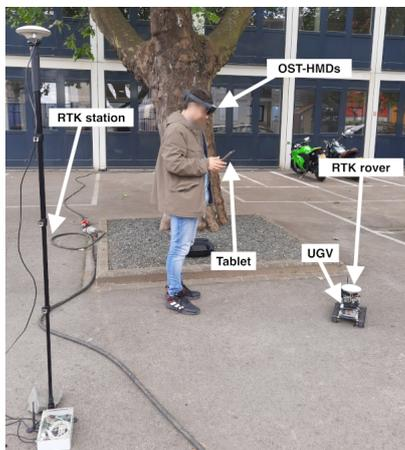
Figure 5: A prototype consisting of a UGV, RTK rover (including an antenna, Swift Navigation Piksi board, and Radio board), RTK station, tablet with a specific application enabling users to remotely command the UGV's movements, and OST-HMD such as the HoloLens v2.
