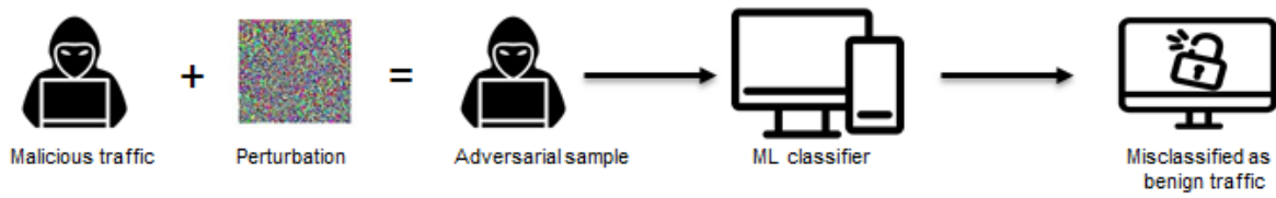
Figure 1: Adversarial attack generation in Network Intrusion Detection System (NIDS) (Jmila and Khedher, 2022).
