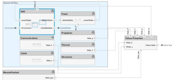
Figure 3: The connection of the failure prediction block with subsystems.
