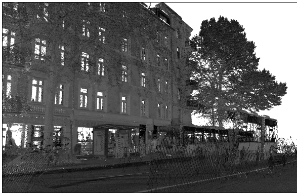
(a) Rendering of a point cloud via rasterization of point primitives. The only available attribute of reflectance intensity is interpreted as a single-channel color.
