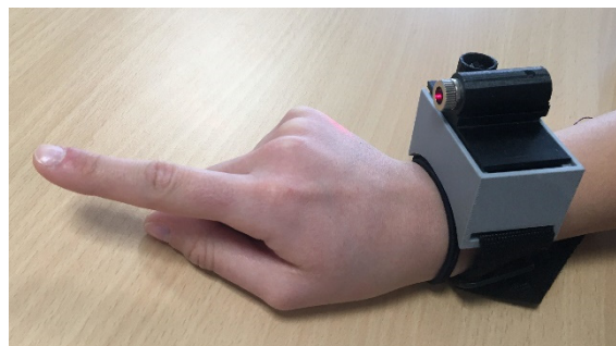
Figure 2: A picture of the wristband integrating the vibration motor and the laser pointer.
