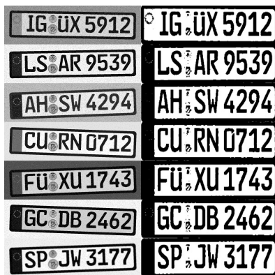
Figure 3: Examples of License Plate Images and Their Representation After Pre-Processing.
