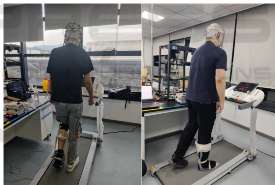
Figure 1: Subjects wearing laboratory-developed powered ankle exoskeleton and unpowered ankle exoskeleton, AFO.
