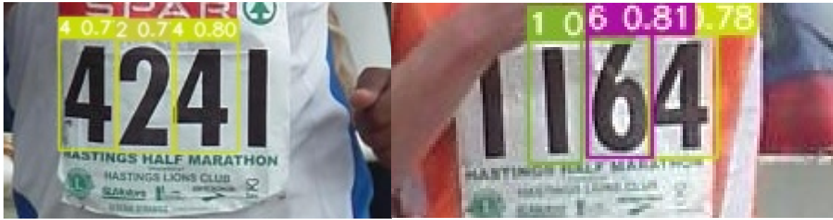
Figure 5: Partially recognized bib numbers, just three digits of four were detected by the digit detector in both samples. The previously adopted metric considers both cases as FPs. A metric evaluating the digit recognition performance provides a better insight into the approach validity.
