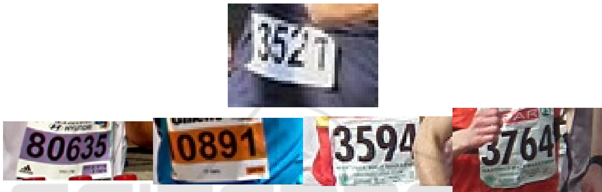
Figure 6: Images that reported a digit FP according to RBNR ground annotation. Upper row: the YOLOv7 digit detector confused a 3521 with 3527. Second row: bibs annotated as 80653, 891, 359, and 764 were recognized as 80635, 0891, 3594, and 3764, respectively. Indeed, those recognized bibs must be considered correct.
