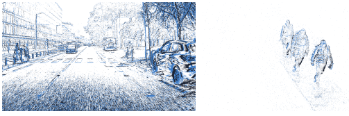
(a) Example recorded with the DVS in motion (b) Example recorded with a stationary DVS
