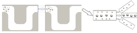
Figure 1: Separation of cells of different sizes based on the use of a periodically repeating curved channel with round edges in the shape of an "S".
