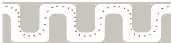
Figure 11: Three S-shaped channel passes of the largest solid two-in-line cluster in the geometry of 160 \times 80 \mu\text{m} at the highest velocity of Re = 64 . One cell out of two is marked in red to better observe the movement, especially the rotation of each cell in the cluster.
