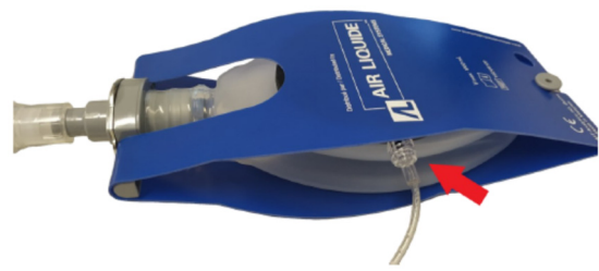
Figure 5: The measuring balloon is inserted inside the artificial lung.
