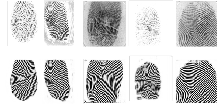
Figure 3: Degraded (top row) and Enhanced (bottom row) image pairs on FVC dataset from enhancement pre-training.
