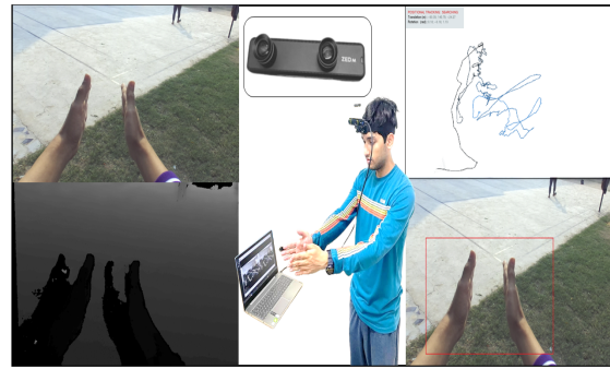
Figure 1: (Middle) Recording platform (A subject with a head-mounted camera for capturing the hand gestures), RGB (left-top) and depth (left-bottom) images generated by the ZED camera, trajectory (Right top) and bounding box labels (Right bottom).
