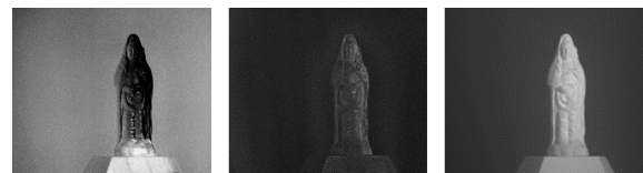
Figure 9: Results of separation of reflection and scattering components: fog first-order scattering (left), specular reflection (center), diffuse reflection + complex scattering (right).
