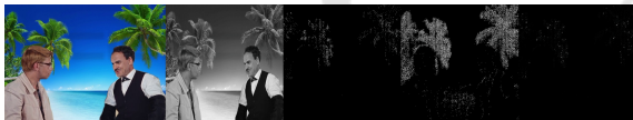
Figure 2: Preprocessing example. At the first step, the original image is converted into the YCbCr format and the preprocessing described above is applied. In the second step, the 2D discrete wavelet brightness transformation is applied. In the third step we calculate the MAD value for each block. In the final step we subtract the MAD value from the second step result.
