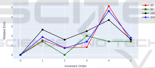
Figure 11: Stability study of Zernike invariants under rotation.
