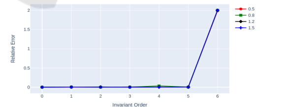
Figure 16: Stability study of Hu invariant moments under scale factor.
