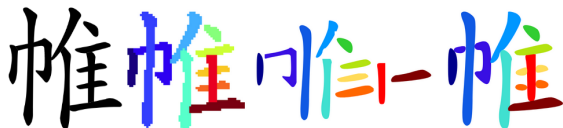
Figure 3: Vectorization by segmenting each stroke instance of a line drawing. Left to Right : Grayscale raster image; segmented output of raster image; instances separated and vectorized, relative position is intentionally modified for visualization purposes; final vectorized result.
