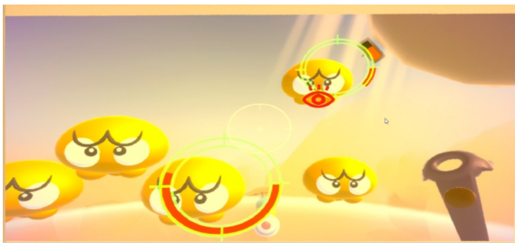
Figure 8: Implementation of a game user interface that presents the gazing point and gazing duration.
