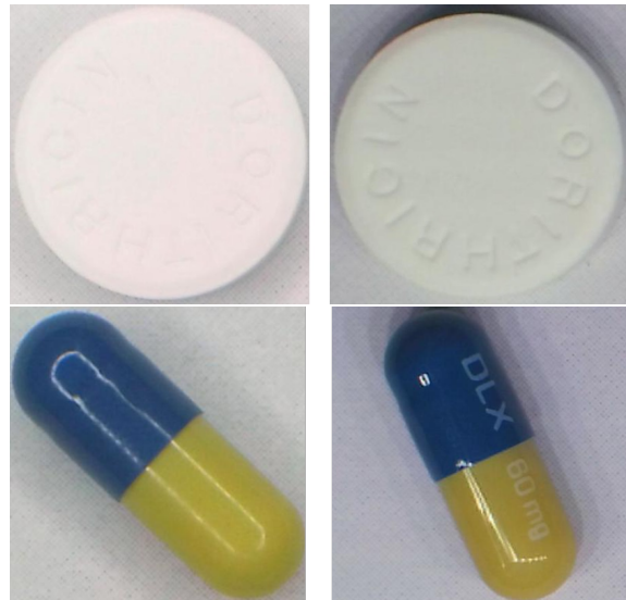
Figure 1: Pill images are captured with different lamps. First line: engraved text is only visible with side-light. Second line: same pills but with different poses, where the white imprint is only visible in the right photograph.
