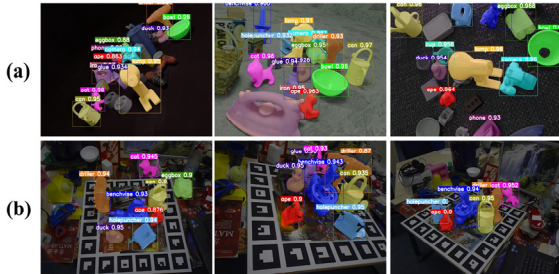
Figure 8: Typical panoptic segmentation results of the proposed approach applied to (a) PBR-synthetic and (b) LMO datasets.
