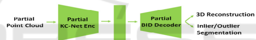
Figure 5: The proposed outlier removal network segmenting a partial point cloud into inlier and outlier clusters.
