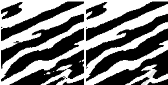
Figure 6: Left: Raw thresholded image. Right: Thresholded image after removing small areas.
