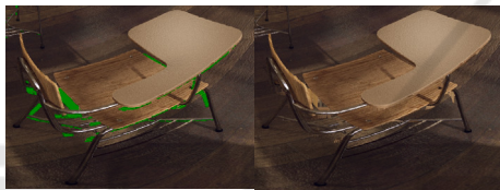
Figure 2: Idea of an image inpainting. Both images contain a fragment of a synthesized virtual view. Left – a direct result of a view reprojection. Right – virtual view inpainted in order to conceal the presence of missing pixels.
