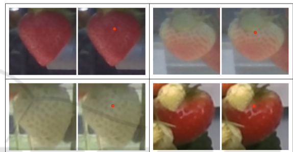
Figure 2: Four illustrative examples from the widest region detection dataset. The images are labeled with the X and Y pixel coordinates of the widest region, indicated by the red dots in the images.
