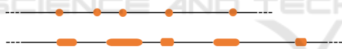
Figure 1: Expansion when moving from a point to an interval process. The finite durations expands the time scale, reducing the operational frequencies.
