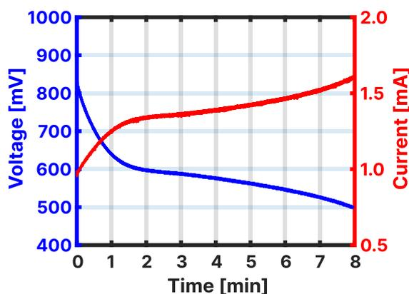
Figure 6: The output voltage and output current response of printed harvesting electrodes.
