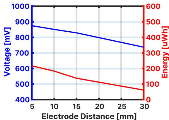
Figure 5: The effect of inter-electrode distance on the harvested energy and voltages.
