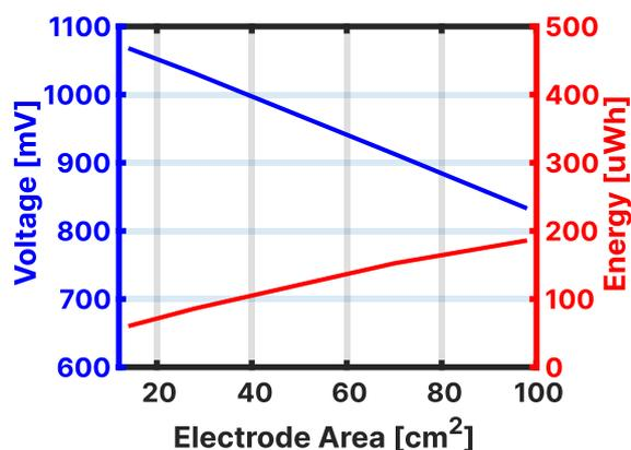
Figure 4: The effect of surface area on the harvested energy and voltages.
