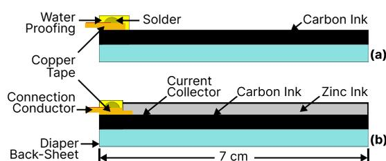
Figure 1: Printed electrode design for energy harvesting; (a) carbon ink cathode, (b) zinc ink anode over the current collector layer of carbon ink.
