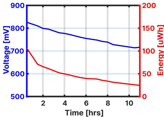
Figure 7: The harvested energy and voltages of the printed electrode over a longer time in the electrolyte.
