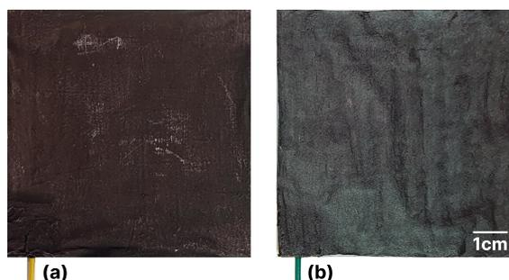
Figure 2: Fabricated flexible harvesting electrodes on diaper back sheets; (a) carbon ink cathode, (b) zinc ink anode.
