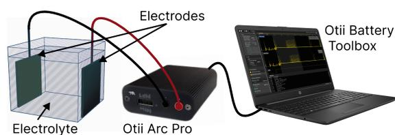
Figure 3: Measurement setup to harvest energy from pseudo-urine.
