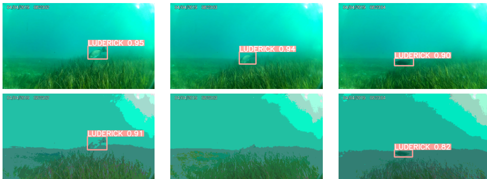
Figure 6: An instance of failure with the encoded dataset. Top row: detections on the raw dataset. Bottom row: corresponding detections on the encoded dataset. The text near the bounding box states the class (luderick) and the confidence score assigned by YOLO.
