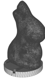
Figure 5: 3D mesh of the inspected object. This model was adopted in our simulation and was used to 3D-print the object on which real-world experiments (i.e., scanning) in the lab were conducted.
