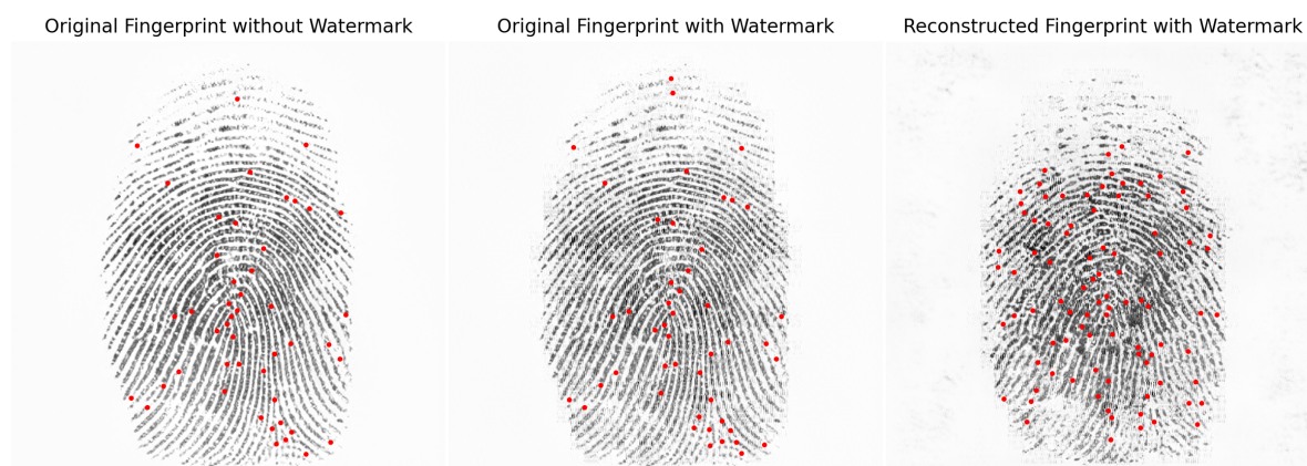
Figure 5: Visualization of a fingerprint image with and without a watermark. The red dots in the figure denote the locations of minutiae.
