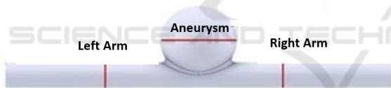
Figure 2: Schematic representation of the locations of the biomodel in which there were taken measurements to evaluate the geometric structure.
