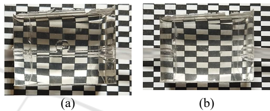
Figure 4: Evaluation of the optical transparency of the biomodel, in which the inlet and outlet channels have an angle of 180° to each other, and where the mold used consisted of polysmooth, for the situation in which the fluid used was water (a) and for the case where the fluid was a glycerin-based solution (b).
