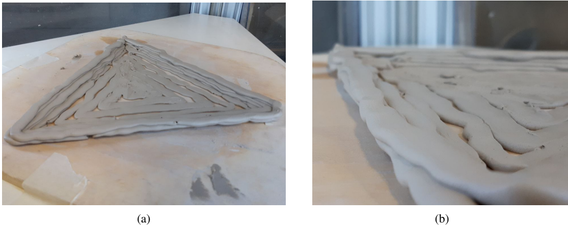
Figure 6: Preliminary example of a clay pot produced using a 3D printer.
