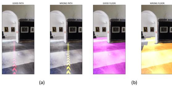
Figure 1: (a) An example of correct (left) navigation instructions and misleading instructions (right) due to the misalignment of the internal navigation map with respect to the real environment. (b) The floor segmentation map according to the internal representation of the navigation system in the two cases. As can be seen, the misalignment between the floor segmentation and the RGB image is an informative signal for world-map misalignment detection.
