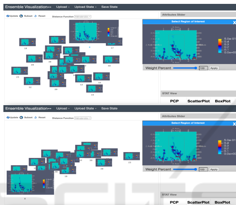
Figure 8: Spatial Region of Interest (ROI) Selection: a) The scientist was interested in exploring a certain region within the reservoir, so s/he selected the ROI and increased its importance over other regions in the grid by 100%. b) The ensemble members are re-projected based on the newly updated weight vector.
