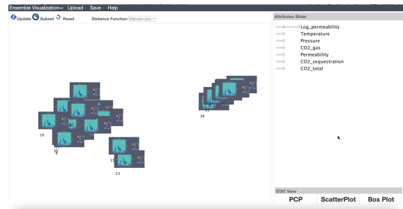
Figure 6: Performing a PLI to investigate the effect of increasing the log permeability weight on the ensemble. The resulted projection led to the conclusion that low permeability in the conductive fracture shallow depth keeps fluid pressure high and prevents CO2 from undergoing phase change to CO2 gas.
