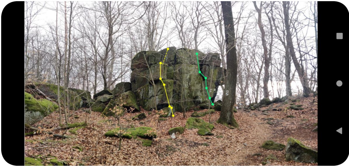
Figure 1: Real-time 3D Information Visualization on Mobile Devices: two polylines rendered as a camera preview overlay with their full visibility indicated with solid lines and partial visibility with a dashed line.
