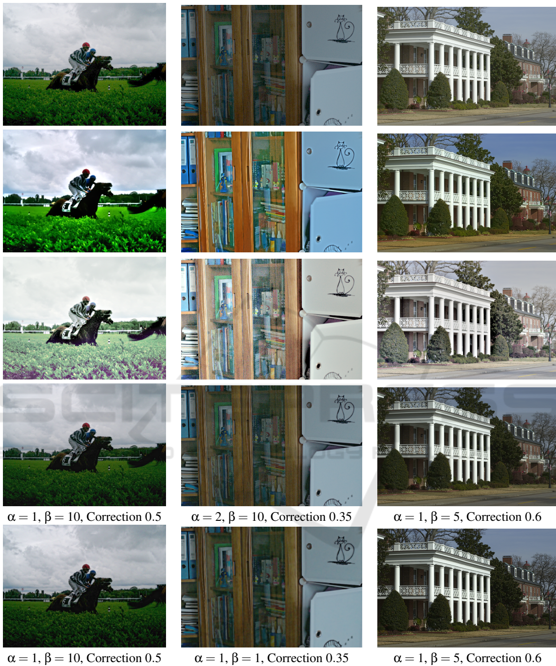
Figure 4: Comparison between state-of-the-art techniques for low-light image enhancement and our models combined with a gamma correction to the illumination component. Each row contains the results by Kimmel et al., LIME, MSR, our Tychonoff model (2), and our TV model (3). Compared to our proposals, the method by Kimmel et al. produces similar results in terms of illumination, but is more sensitive to noise, LIME produces oversaturated colors, while MSR is not robust to noise and exhibits color issues. Our methods provide a good compromise between discounting the illumination, avoiding the amplification of noise, and preserving color and geometry. Note also that the results by Tychonoff are slightly more blurred than those of TV, as seen in the clouds and grass of Horses and on trees on Building .
