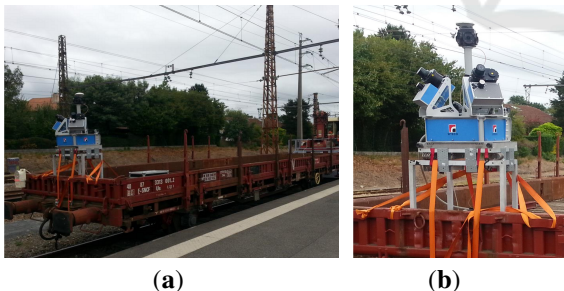
Figure 1: Experimental platform: (a) overview of the wagon, (b) acquisition device.
