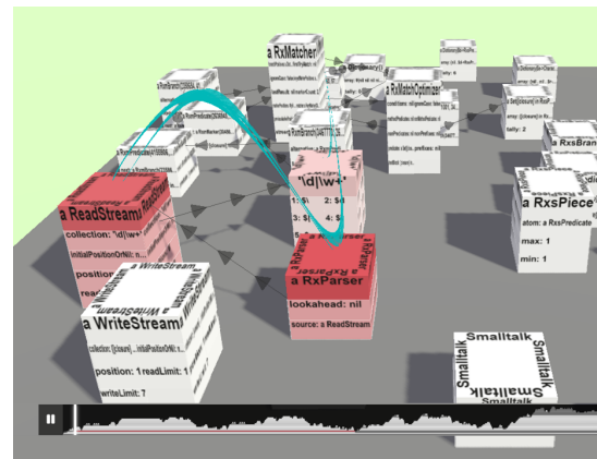
Figure 1: Screenshot of an animated object map showing a program trace for the construction of a regular expression matcher in the Squeak/Smalltalk programming environment. Blocks represent objects, arrows display references between objects, and color highlights and trails show object activations. The timeline at the bottom provides a temporal overview of the program trace.
