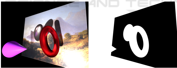
Figure 8: The left image shows a randomized scene. The right image shows the same scene after changing the plane to a diffuse black and changing all geometric objects to a diffuse white color. The rendered image is binary.
