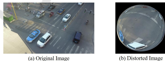
Figure 1: Example of pronounced distortions in a fisheye image, particularly near the edges.
