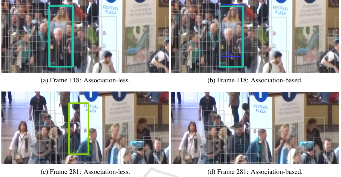
Figure 3: Our proposed association-less track management from Eq. (15) vs. traditional association-based track management on “MOT20-07”. Select tracks are highlighted in color based on track-ID, while boxes of unrelated tracks are drawn in gray. In crowded areas, the detector tends to generate clutter detections, which can lead to false tracks, as in Fig. 3b. Meanwhile, detections of partially occluded objects tend to have low confidence, which can cause the tracker to require more frames before a track is established, as in Fig. 3d. Our association-less track management enables the tracker to be conservative in establishing tracks in crowded areas, and at the same time aggressive for solitary objects. Meanwhile, association-based track management must more carefully balance the risk of false tracks and delayed track establishment.
