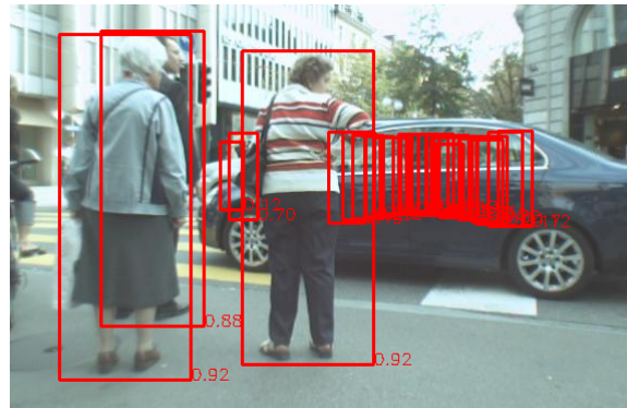
Figure 4: An image from “MOT17-05-FRCNN” processed using the pretrained detector from ByteTrack (Zhang et al., 2021). This detector is overfitted to “see through” severe occlusions, resulting in a large number of clutter detections.
