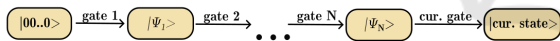
Figure 3: Schematic of the sequential application of the updated list of actions on the initial state |00..0\rangle transforming it to the current state outputted by the environment.
