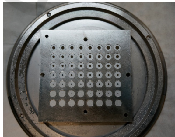
Figure 1: Coated calcium fluoride substrates on the sample plate after the pulsed laser deposition coating process, with the front plate and the coating mask removed.
