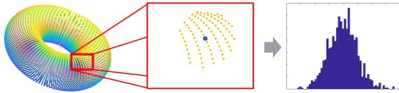
Figure 4: Creating a histogram of reflection intensity, after selecting points within a specified radius from the focal point and creating a local point cloud, the reflectance intensity of points contained in this local point cloud is the subject of the histogram.
