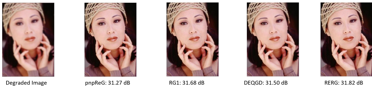
Figure 1: Image results for the GD based methods with corresponding PSNR in dB.
