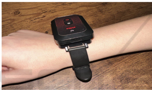
Figure 1: The RTLS tag mounted on the GT9X Link wristband worn by a participant.
