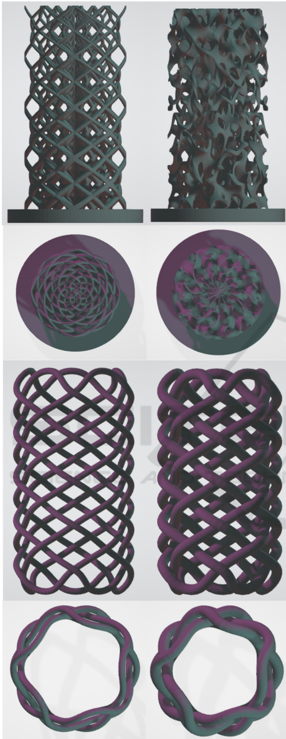
Figure 3: Topology optimized and functionally graded tissue engineering scaffolds (upper images). Algorithmic design of woven meshes for stent-like medical devices with improved mechanical compliance (lower images).
